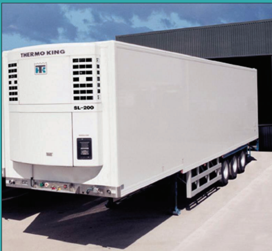
Thermo Kings SL200e transport refrigeration system mounted to a refrigerated trailer.
